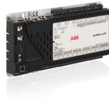
Compact motion controller with real-time Ethernet POWERLINK technology
